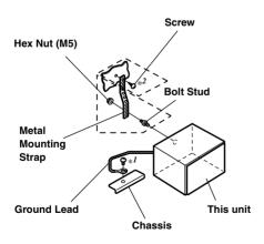
Reinforce the head unit with the metal mounting strap (not supplied). Secure the ground lead of the unit to a clean metal spot using a screw ( $^{*I}$ ) already attached to the vehicle's chassis.
